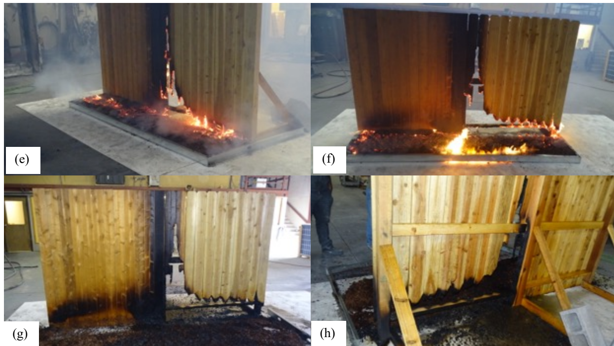
Figure 2. Test 1 showing (a) ignition – 0 min, (b) fan on – 30 s, (c) burning east board – 6 min, (d) open section – 11 min, (e) flame propagation – 18 min, (f) near end of test – 29 min, (g) after test, and (h) back of fence.
